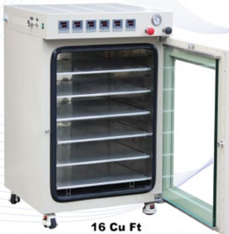
AccuTemp-160 25.5x30.5x35.5" vacuum ovens with 6 heated shelves/sensors/controllers, all st. vacuum tubing, oil-filled vacuum gauge, secondary over-temp dial, built-in LED light, vacuum and vent ports with needle valves, 3rd gen low-temp controller, and adjustable gas back-fill capability
