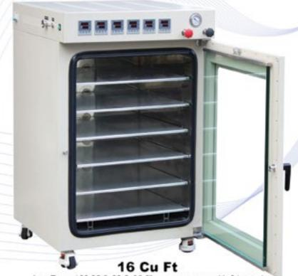
AccuTemp-160 25.5x30.5x35.5" vacuum ovens with 6 heated shelves/sensors/controllers, all st. st. vacuum tubing, oil-filled vacuum gauge, secondary over-temp dial, built-in LED light, vacuum and vent ports with needle valves, 3rd gen low-temp controller, and adjustable gas back-fill capability.
